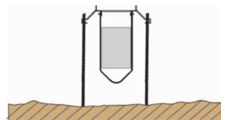
9812 using rebar in installation brackets
